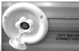
City Water Fill with City Water Connection Label
